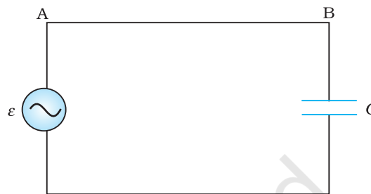
FIGURE 7.8 An ac source connected to a capacitor.
